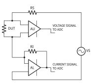
Voltage across the component is generated by the test signal source Vs. Both the amplitude and frequency of Vs can be set. The voltage is applied to the device under test (DUT) through the source resistance Rs. Current flows to the virtual ground of the current amplifier AI, and through the current conversion resistor Ri. The output of AI provides a signal proportional to the current, I\*Ri.
