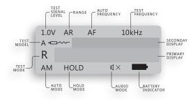
**PRIMARY DISPLAY:** The Primary Display is located in the middle of the screen and uses the largest font. It shows the dominant impedance parameter reading typically with 5 digits displayed.
